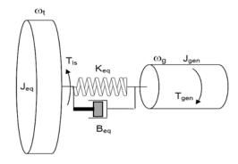
Figure 6. Case II Gear System: Two Masses
