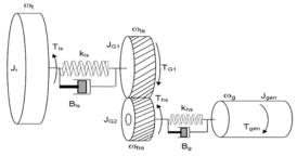
Figure 5. Case II Gear System: Three Masses
