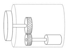
Figure 3. Typical Gear System of Wind Turbine
