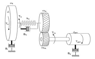
In particular, most controllers are considered more adapted for high-flexibility wind turbines that cannot be properly modeled with a one mass model [8]. Besides, it is shown that [9] the two-mass model can show flexible modes in the gear train model that cannot be done using the one mass model. Besides, this model was also used to investigate the linear and the nonlinear controller of the wind turbine [10]. The essential assumptions of the present model are:
