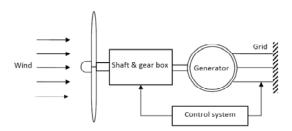
Figure 1. Components of a Typical Wind System
